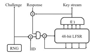
Figure 2: Crypto-1 stream cipher and initialization.
