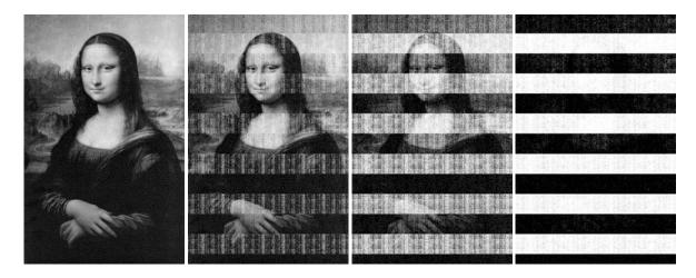
Figure 4: We loaded a bitmap image into memory on Machine A, then cut power for varying lengths of time. After 5 seconds (left), the image is indistinguishable from the original. It gradually becomes more degraded, as shown after 30 seconds, 60 seconds, and 5 minutes.
