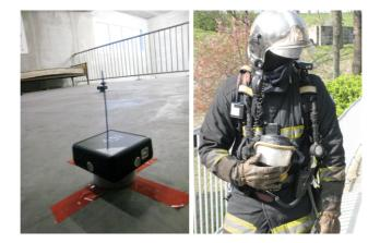
Figure 1: A first generation RELATE sensor node placement on the floor of the training facility and a firefighter equipped with several sensor nodes
