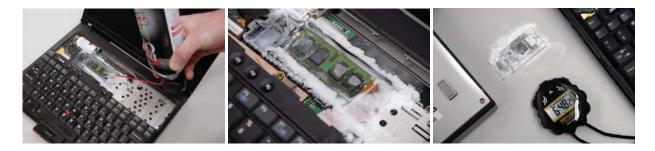
Figure 5: Before powering off the computer, we spray an upside-down canister of multipurpose duster directly onto the memory chips, cooling them to -50 °C. At this temperature, the data will persist for several minutes after power loss with minimal error, even if we remove the DIMM from the computer.
