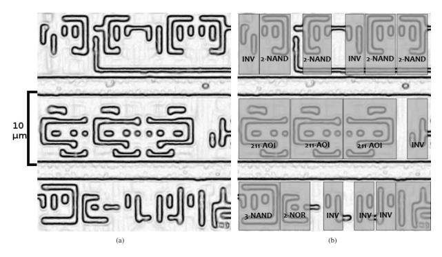
Figure 1: (a) Source image of layer 2 after edge detection; (b) after automated template detection.
