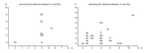
**Fig. 1.** Success rate of jamming depending on the position of the attacking mote. The Tx and Rx labels are the transmitting and receiving motes. The numbers 0–100 in the graphs denote the percentage of packets that were jammed when the attacking mote was in that 2D position relative to Tx and Rx (section 4.3).
