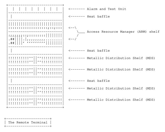
The SLC-2000 RT is a modular design usually consisting of the following components:
