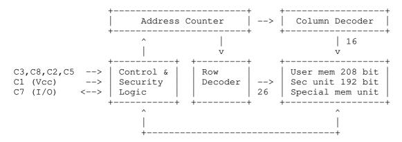
The SLE4404 memory is subdivided in three main memory blocks: one is read only (a "PROM" containing the manufacturer code and/or a serial number and an expiration date), the second is both readable and writeable (user memory) and the last block cannot be written to unless the lock-out fuse has been fused.
