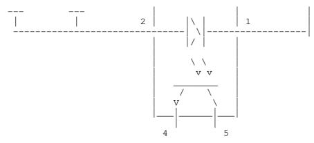
Pins 4 and 5 on the optical coupler can be wired to remotely start a device upon answering the line. An example would be a tape machine or batterypowered bugging amplifier. Be careful not to connect anything over 25 volts to pins 4 and 5 to avoid frying the opto-coupler. Either circuit will accommodate an extra LED that could be used as a status indicator. Just be sure to keep the polarity proper and put it in series with the other components.
