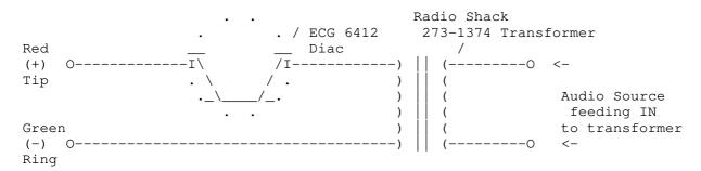
The "Diac" or "Bilateral Trigger Diode" looks like an open circuit until a voltage of either polarity is applied that is above its threshold of 63 Volts. (plus or minus 7 Volts) When this voltage is exceeded, like when the line rings, the device acts as a switch and goes into conduction. This "answers" the phone and holds the line through the transformer, which couples the audio to the line.
