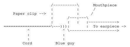
(The paper clip is shoved under the blue guy to make a good connection between the inside of the mouthpiece and the metal cord.)
