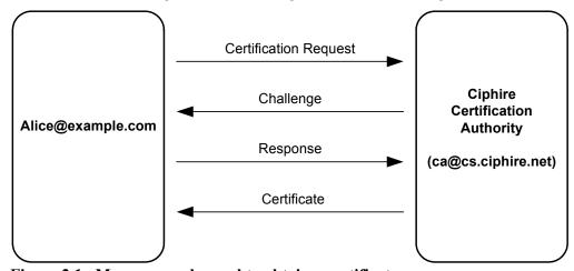
Figure 2.1. Messages exchanged to obtain a certificate.
