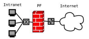
Figure 1: Easy Firewall Model
